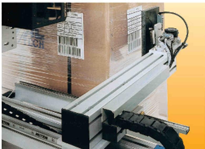
label detector", and a barcode scanner which also detects the presence of the label on the pallet, and will initiate a second cycle to compensate if necessary, or a signal to stop the production line.
