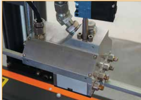
Upper Hot Melt glue dispensing applicator
